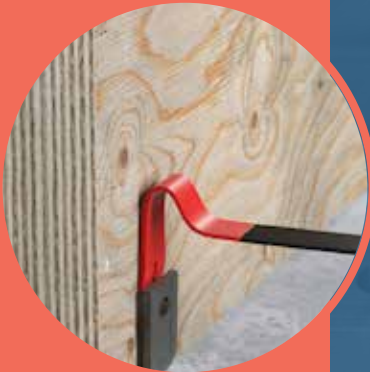
GOUGES, DENTS AND CHIPS FROM CONVENTIONAL FORM CLIP REMOVAL RUINS EXPENSIVE FORMS
