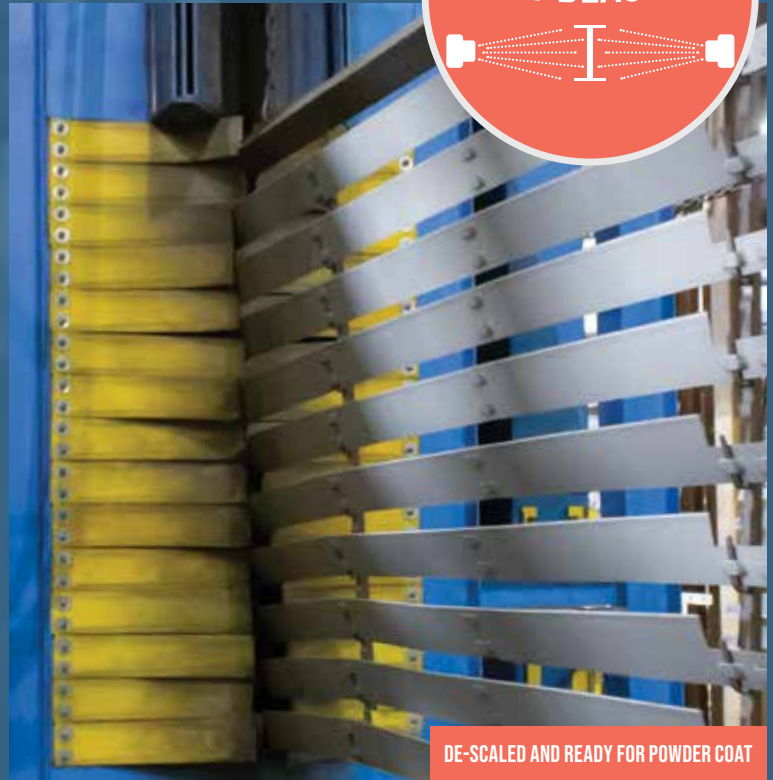
RUSTED MATERIAL ENTERING SHOT BLASTER
