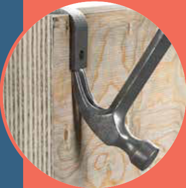
GOUGES, DENTS AND CHIPS FROM CONVENTIONAL FORM CLIP REMOVAL RUINS EXPENSIVE FORMS
