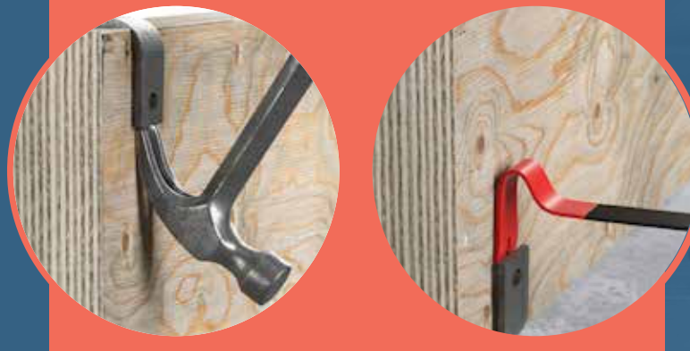
GOUGES, DENTS AND CHIPS FROM CONVENTIONAL FORM CLIP REMOVAL RUINS EXPENSIVE FORMS
