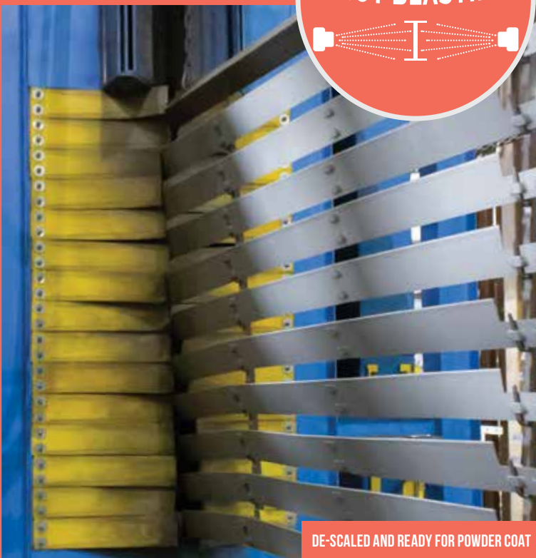
RUSTED MATERIAL ENTERING SHOT BLASTER
